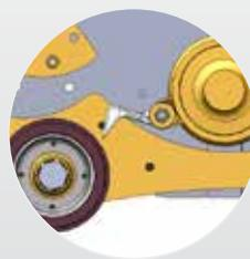
With the roller positioned close to the rotor, it is automatically cleaned by the rotating flails and the cut material is evenly distributed over the top of the roller.
