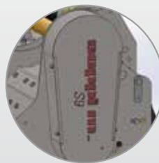
Strong welded belt cover minimizes accidental damage.
