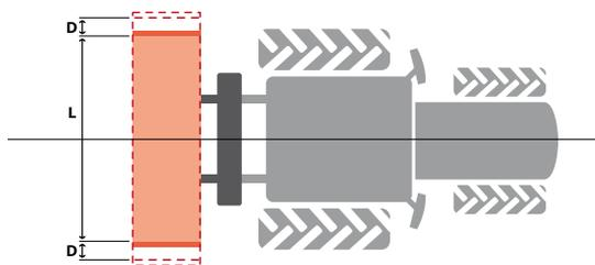
The **WBS fh** can be side shifted by 35 cm [14"], both left and right of the central position.
